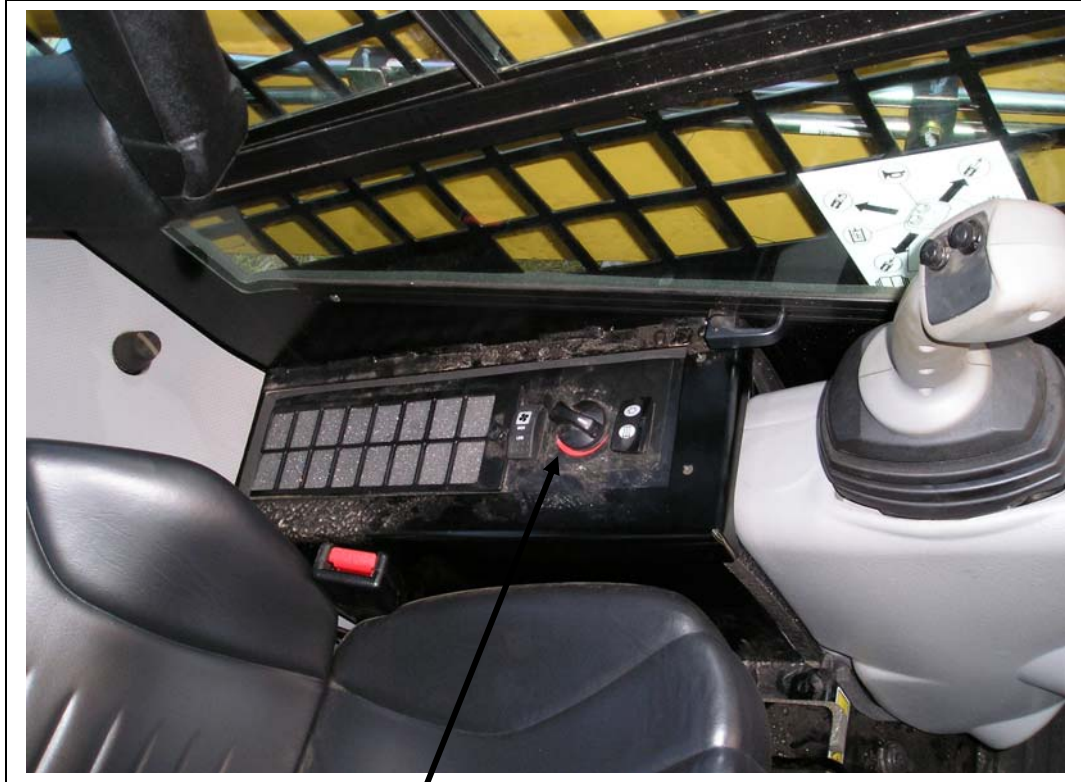
Heater - A/C box in place with cab back down.
